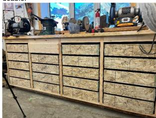
(Using OSB as the foundational construction material has worked out exceptionally well for a shop cabinet.)
