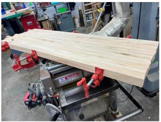
(I am going to glue up the last of the strips that I cut for one last counter. This is exactly how I built the main counter for my new shop cabinet.)
