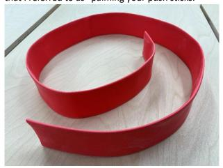
(This is the heat shrink tubing that I use to secure the magnet in place, mark where the stick should be held and provide a little extra grip.)
