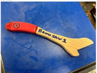
(The "X" marks where the magnet is and this magnet allows the push stick to stick to your machine.)
